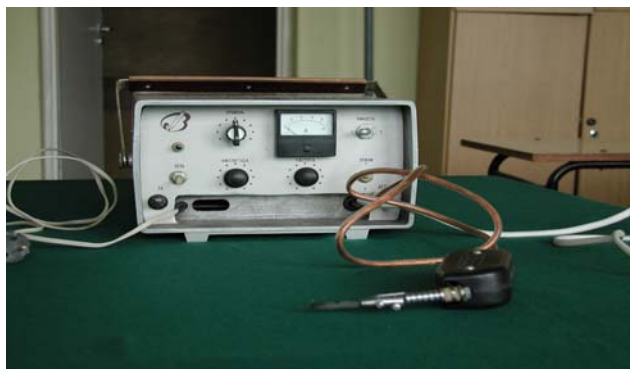
Fig. 1. The equipment used for electro – spark alloying (model EIL-8A)
